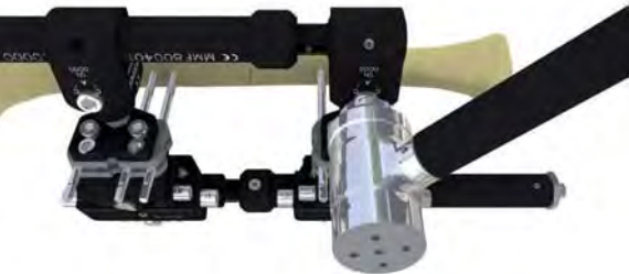
Fig. 14 Tighten the spherical joints on the fixation unit using the appropriate dynamometric wrench on the hexagonal bushes of the supports.
